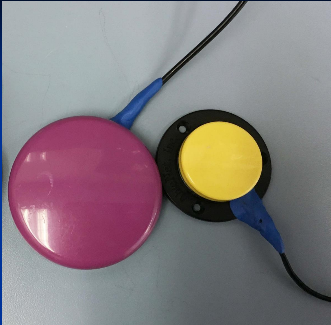
Sugru molded around end of wire to reduce fraying
